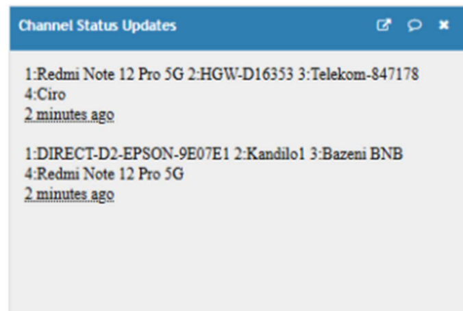
Fig. 4: ThingSpeak channel status log associating detected SSIDs with RSSI fields.
